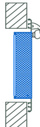
Hinged insulated Control Cover
