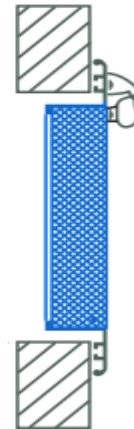
Hinged insulated Control Cover
